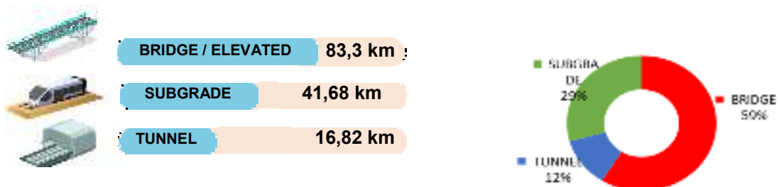
Figure 2. The main work of the Jakarta Bandung high-speed railway project
